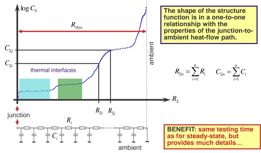
The structure function illustrates the way how heat flows though a package.
