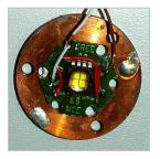
— MCPCB-s made of Al and Cu, heat-slug soldered
