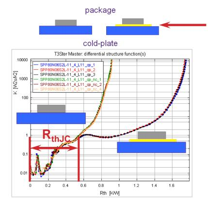
Change the quality of the thermal interface Measurement of 2 setups (2x3
