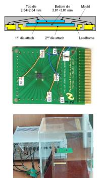
Majority of the  $R_{thja}$  is caused by the JEDEC standard test environment.
