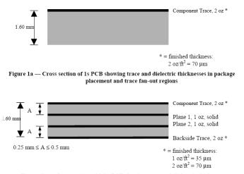
Figure 1b — Cross section of 2s2p PCB showing trace and dielectric thicknesses
