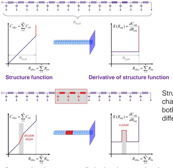
Structural or material property changes are clearly indicated both by the cumulative and the differential structure functions
