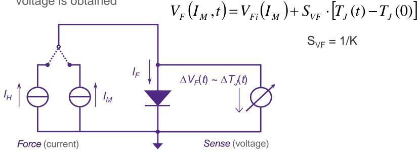
Forward voltage change due to temperature change is measured using a 4 wire setup (Kelvin setup)
