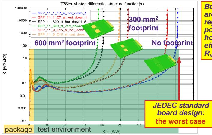
Board design (Cu area of footprint region) and board position (vertical or horizontal) strongly effects the ultimate R<sub>thja</sub> value
