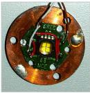
MCPCB-s made of Al and Cu, heat-slug soldered
