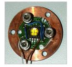
FR4 PCB, heat-slug soldered to the Cu block
