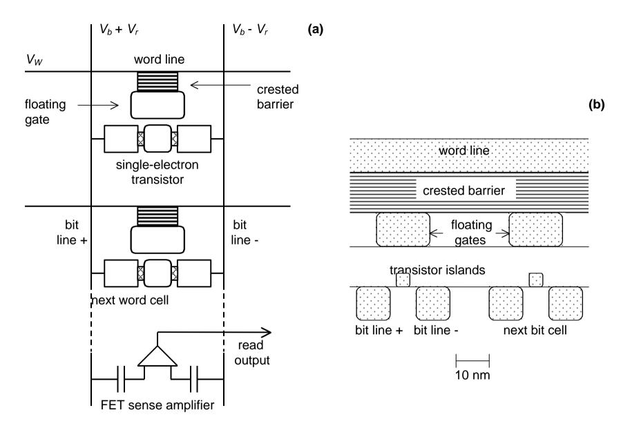
Fig. 14. Hybrid SET/FET memory insensitive to the background charge randomness: (a) schematics, and (b) side view on a possible layout compatible with room-temperature operation and a density of 100 Gbits/cm<sup>2</sup>. (After Ref. 164.)
