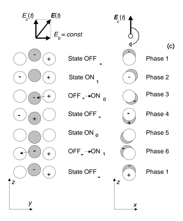
Fig. 11. SET Parametron: (a) schematics and (b) energy diagram at 3 values of the clock field  $E_c(t)$ . Energy difference  $\Delta$  between the edge islands is proportional to the signal field  $E_s$ , while the energy shift W(t) of the middle island is determined by the clock field. (c) Shift register using a variety of SET Parametron cells ("single-exciton parametrons") which do not require the initial charging. (After Ref. 142).
