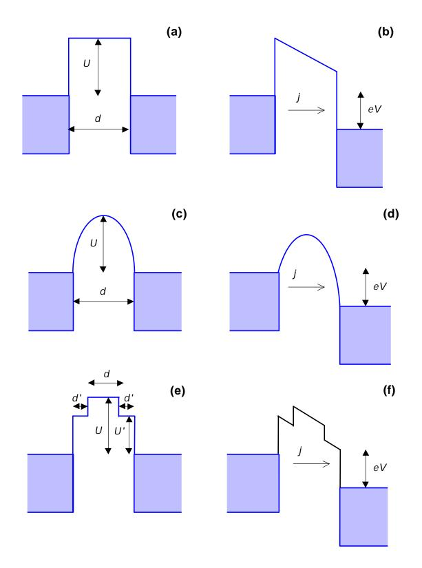
Fig. 15. Various tunnel barriers without (left column) and with (right column) applied electric field: (a, b) Usual uniform barrier (often called "rectangular" or "trapezoidal"). (c, d) Crested barrier with parabolic profile. (e, f) Trilayer crested barrier. (After Ref. 167.)
