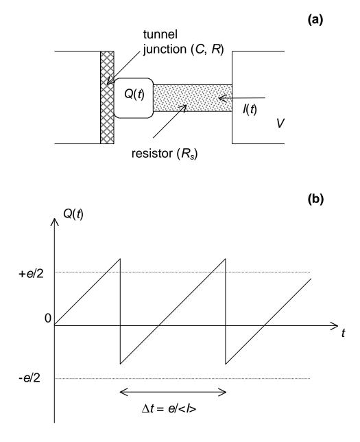
Fig. 9. The simplest single-electron oscillator: (a) schematics and (b) typical dynamics of the tunnel junction charge.
