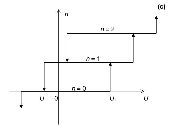
Fig. 7. Single-electron trap: (a) schematics, (b) electrostatic energy of an extra electron as a function of its position for three values of the gate voltage U, and (c) the static characteristic of the device (at  $T \rightarrow 0$ ).
