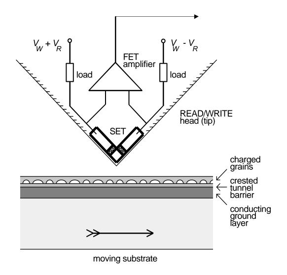
Fig. 21. Proposed electrostatic data storage system with hybrid SET/FET readout. (After Ref. 178.)
