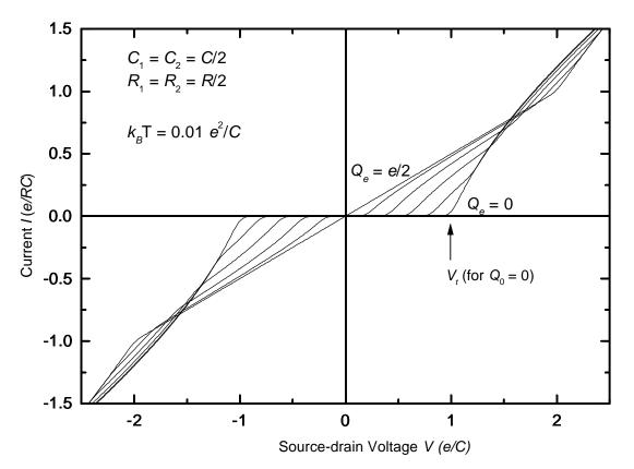
Fig. 6. Capacitively-coupled single-electron transistor: (a) schematics, (b) source-drain dc *I-V* curves of a symmetric transistor for several values of the  $Q_e$ , i.e. of the gate voltage, and (c) the Coulomb blockade threshold voltage  $V_t$  as a function of  $Q_e$  at  $T \rightarrow 0$ .
