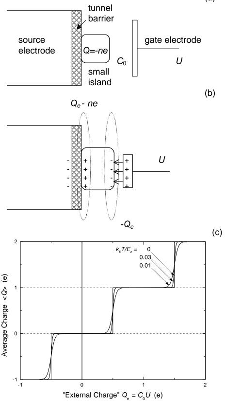
Fig. 5. Single-electron box: (a) schematics, (b) a particular geometry in which the "external charge"  $Q_e = C_0 U$  can be readily visualized, and (c) the "Coulomb staircase", i.e. the step-like dependence of the average charge Q = -ne on the gate voltage, for several values of temperature.
