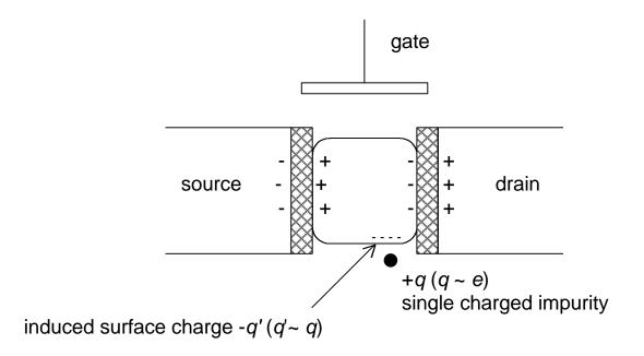
Fig. 12. The effect of a single charged impurity on the single-electron transistor.
