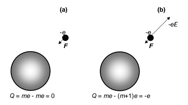
Fig. 1. The basic concept of single-electron control: a conducting island (a) before and (b) after the addition of a single electron. The addition of a single uncompensated electron charge creates an electric field E which may prevent the addition of the following electrons.
