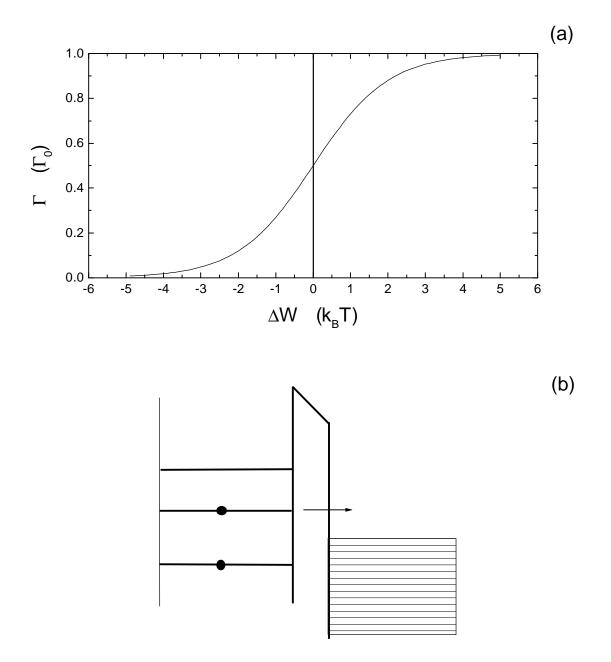
Fig. 4. (a) The rate  $\Gamma$  of electron tunneling from/to a discrete energy level to/from a Fermi-sea continuum according to Eq. (8), and (b) an energy diagram of a tunnel junction explaining why in this case  $\Gamma = \Gamma_0 \approx \text{const}$  at  $\Delta W >> k_B T$  (cf. Fig. 3).
