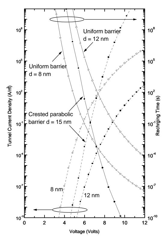
Fig. 16. Tunnel current (solid lines) and floating gate recharging time scale (dashed lines) for usual rectangular barriers with two values of thickness *d* (open points), and for a crested parabolic barrier shown in Fig. 15c,d (solid points). In all cases the maximum height of the barrier U = 3.2 V, and the electron effective mass under the barrier is  $m = 0.3m_0$  (the parameters correspond to a SiO<sub>2</sub> barrier between  $n^+$ -doped silicon electrodes. (After Ref. 167.)
