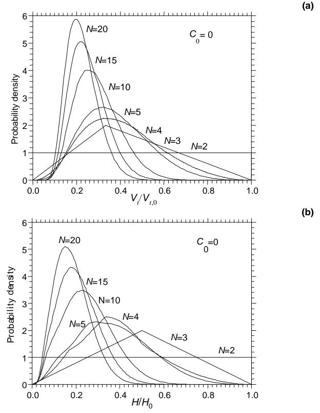
Fig. 13. Histograms of (a) Coulomb blockade threshold voltage  $V_t$ , and (b) energy barrier height H for statistical ensembles of 1D single-electron arrays with N tunnel barriers and random background charges of islands. Index 0 corresponds to the values of  $V_t$  and H in the absence of background charges. All the junction capacitances C are assumed equal, stray capacitances negligibly small. Figure courtesy of Dr. A. Korotkov (unpublished).
