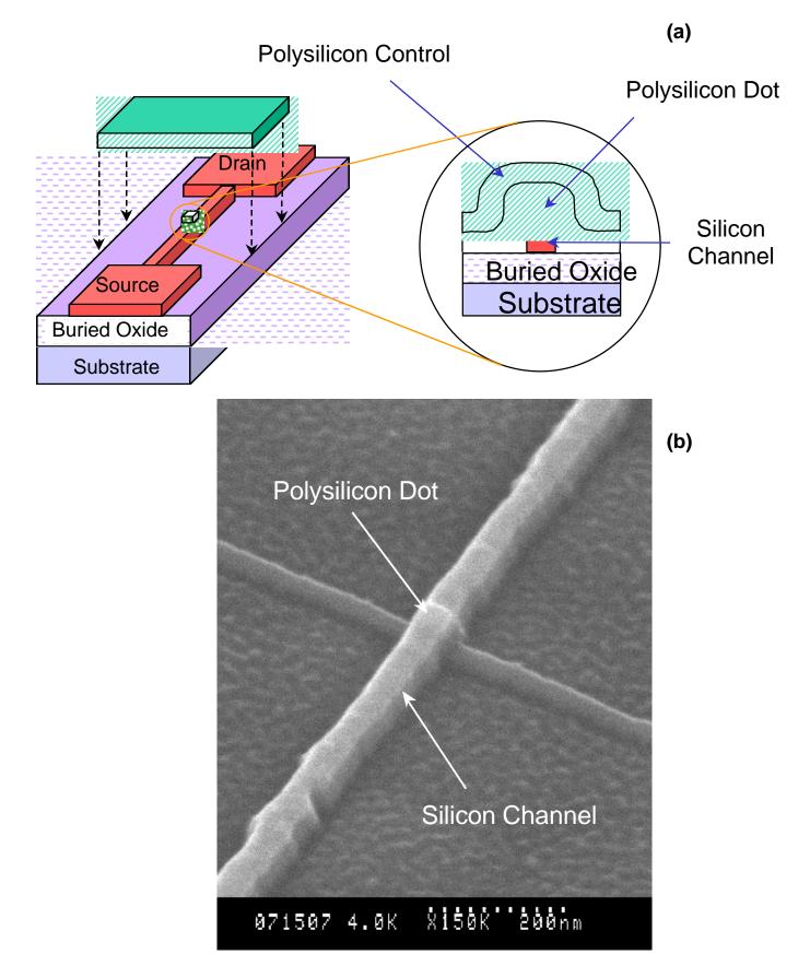
Fig. 19. Floating gate memory cell developed at the University of Minnesota: (a) schematics and (b) SEM picture taken before the control gate deposition. (After Ref. 175.)
