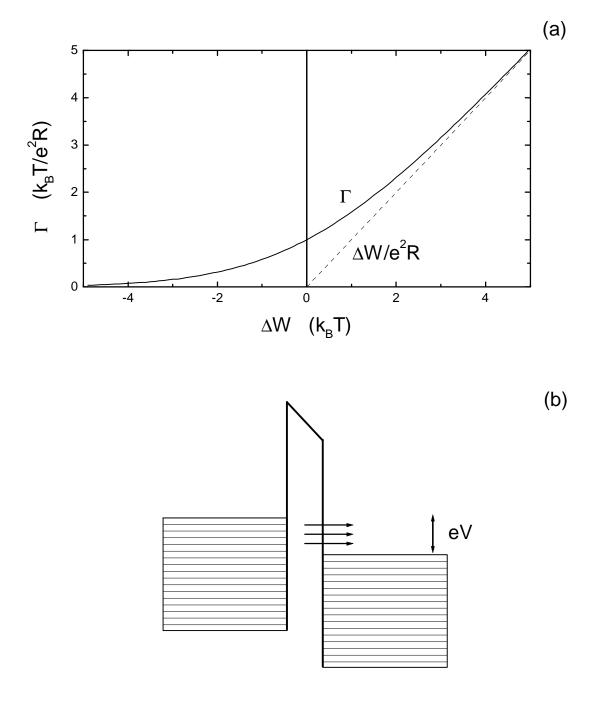
Fig. 3. (a) Single-electron tunneling rate  $\Gamma$  as a function of the electrostatic energy loss  $\Delta W$ , according to Eq. (5) of the orthodox theory, and (b) an energy diagram of a tunnel junction, explaining why  $\Gamma \propto \Delta W$  at  $\Delta W >> k_B T$ : the rate is proportional to the number of occupied quantum states in the electron source, which contribute to the total probability of tunneling into empty states of the collector.
