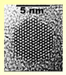
TEM image shows the crystalline arrangement of atoms in a 5 nm CdSe quantum dot particle
