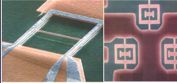
NANOMECHANICAL AMPLIFIER overcomes the vexing probl mofee by providing up to 1,000-fold amplification of weak forces. Two suspended bridges ( left and right ) of monocrystalline silicon carbide support the central crossbridge, to which the signal force is applied Thin-film electrodes [ silver ] atop these structures provide very sensitive readouts of na ioscale motio
