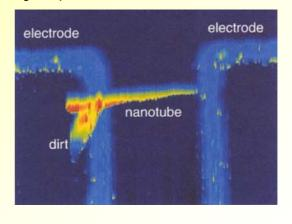
Electrical testing configuration of single electron transistor made out of a nanotube
