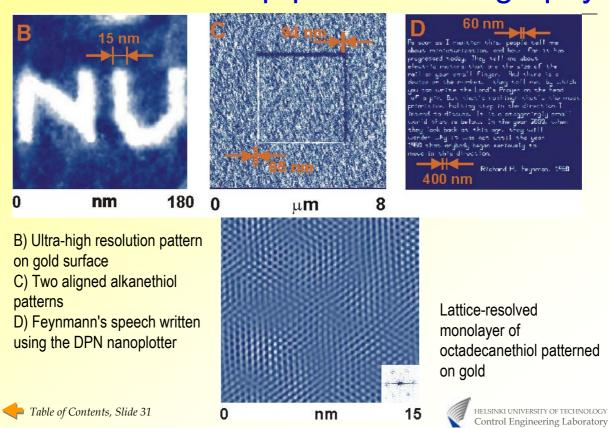
Assembly tool for molecular structures
