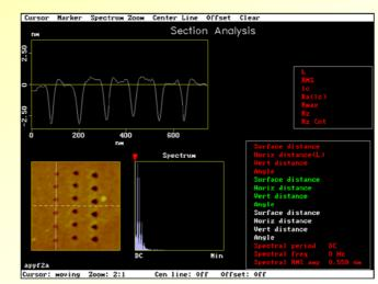
15 nm thick diamond-like carbon film indented 6 times with 3 forces
