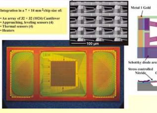
Stored bits: indentations at a "pitch" (distance between centers of neighboring indentations) as high as 40 nm, leading to areal density of ca. 400 gigabits per square inch.
