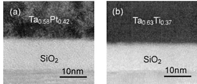
Fig. 2. Cross-sectional TEM micrographs of (a)  $\text{Ta}_{0.58}\text{Pt}_{0.42}/\text{SiO}_2$  structure and (b)  $\text{Ta}_{0.63}\text{Ti}_{0.37}/\text{SiO}_2$  structure after annealing in  $\text{N}_2$  ambient for 30 minutes at 600 °C. No Interfacial reaction are observed.
