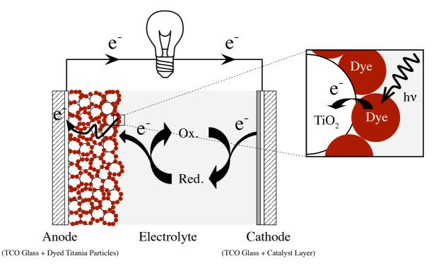
The space left between the two electrodes is filled with an electrolyte that ensures charge transportation through a redox couple. lodide/tri-iodide in a nitrile solvent is typically used for this purpose.
