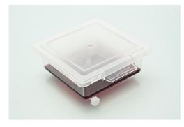
Close the container and wait for the staining to complete. The sensitization process typically takes 4 to 8 hours at room temperature, depending on the titania layer thickness and concentration of the dye solution. Staining can be accelerated by increasing the dye solution concentration if necessary.
