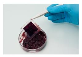
Remove the stained electrode and rinse it carefully with ethanol. Wait a few minutes for the ethanol to evaporate or use a hair-dryer to gently dry the electrode faster.
