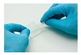
With a rigid squeegee, such as a microscope slide or a glass rod, spread the paste down the plate with the support of the adhesives tape on either side.
