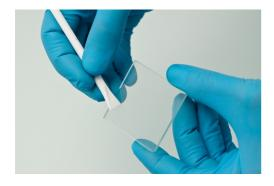
This section focuses on the preparation of the glass substrates for those who would like to prepare their own electrodes from scratch. It includes cutting the glass to the desired size and gives advice for cleaning prior to making any deposition.
