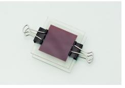
**Hint:** Room for Contacts It is very convenient to slightly shift the glass plates to leave room for the contacts.
