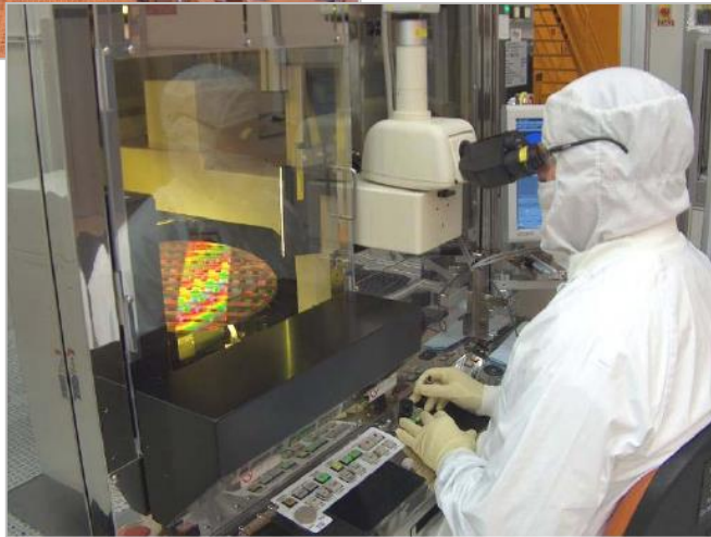
An Intel manufacturing technician uses a scanner to start the very first 45nm production lot of 300mm wafers inside of Fab 32, Intel's first high-volume 45nm chip factory in Chandler, Ariz.
