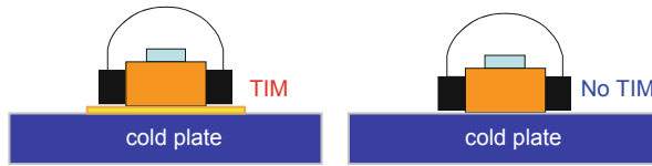
Fig. 4.31 Sketch of the two boundaries: with TIM layer (“wet” condition) and without TIM layer (“dry” condition)
