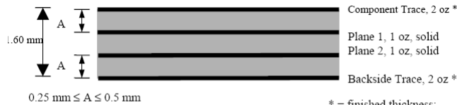
Figure 1b — Cross section of 2s2p PCB showing trace and dielectric thicknesses
