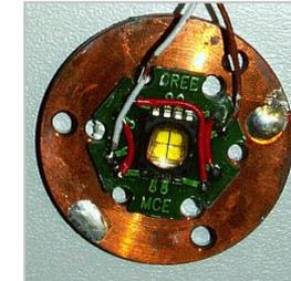
— MCPCB-s made of Al and Cu, heat-slug soldered
