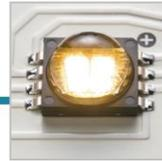
— FR4 PCB, heat-slug soldered to the Cu block
