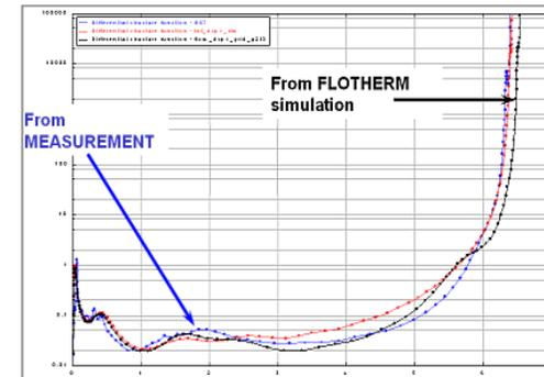
**Structure functions** for test based compact model generation
