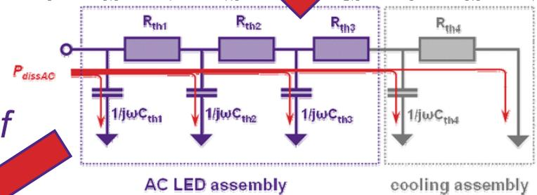
$$Z_{th}(\omega) = \frac{1}{j\omega C_{th1}} \times \left\{ R_{th1} + \frac{1}{j\omega C_{th2}} \times \left( R_{th2} + \left[ \frac{1}{j\omega C_{th3}} \times \left( R_{th3} + Z_{th-cooling\_ass} \right) \right] \right) \right\}$$
