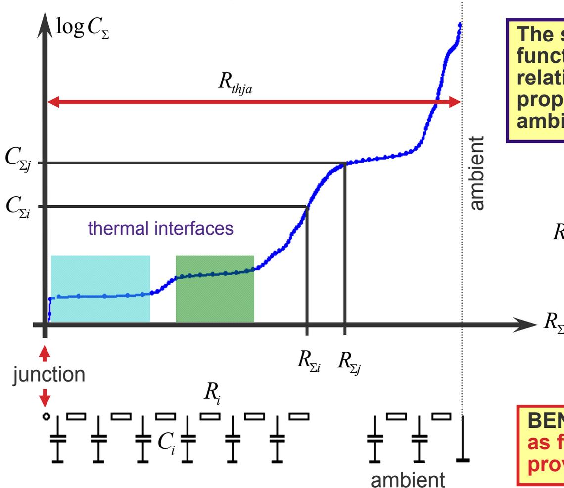
The shape of the structure function is in a one-to-one relationship with the properties of the junction-to-ambient heat-flow path.
