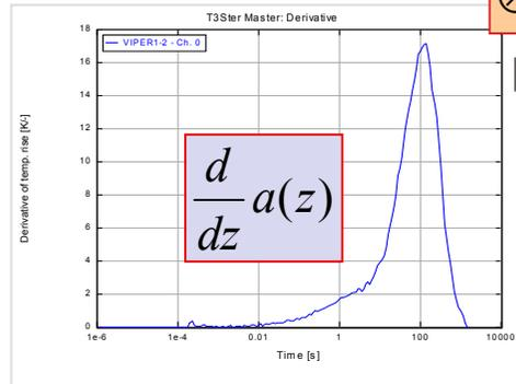
Derivative of the thermal impedance curve
