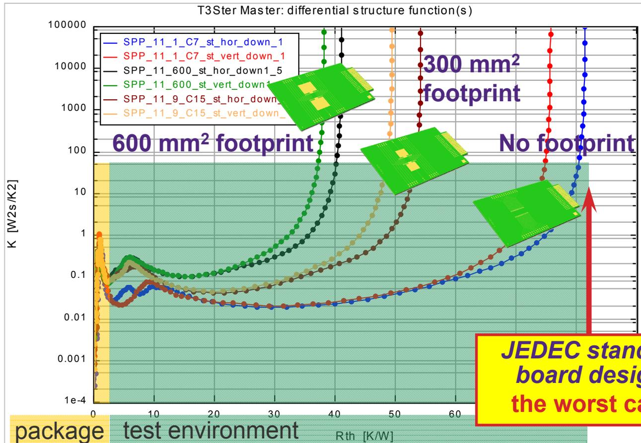
**Board design (Cu area of footprint region) and board position (vertical or horizontal) strongly effects the ultimate  $R_{thja}$  value**
