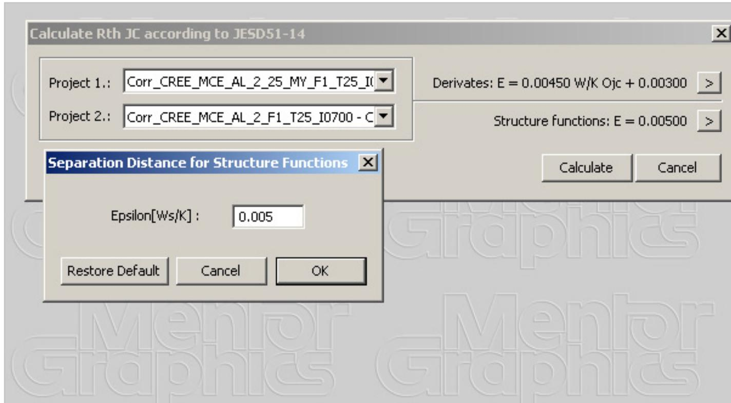
Settings when  $R_{thJC}$  is to be calculated from the **structure functions**. Default would usually do.
