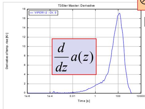
Derivative of the thermal impedance curve
