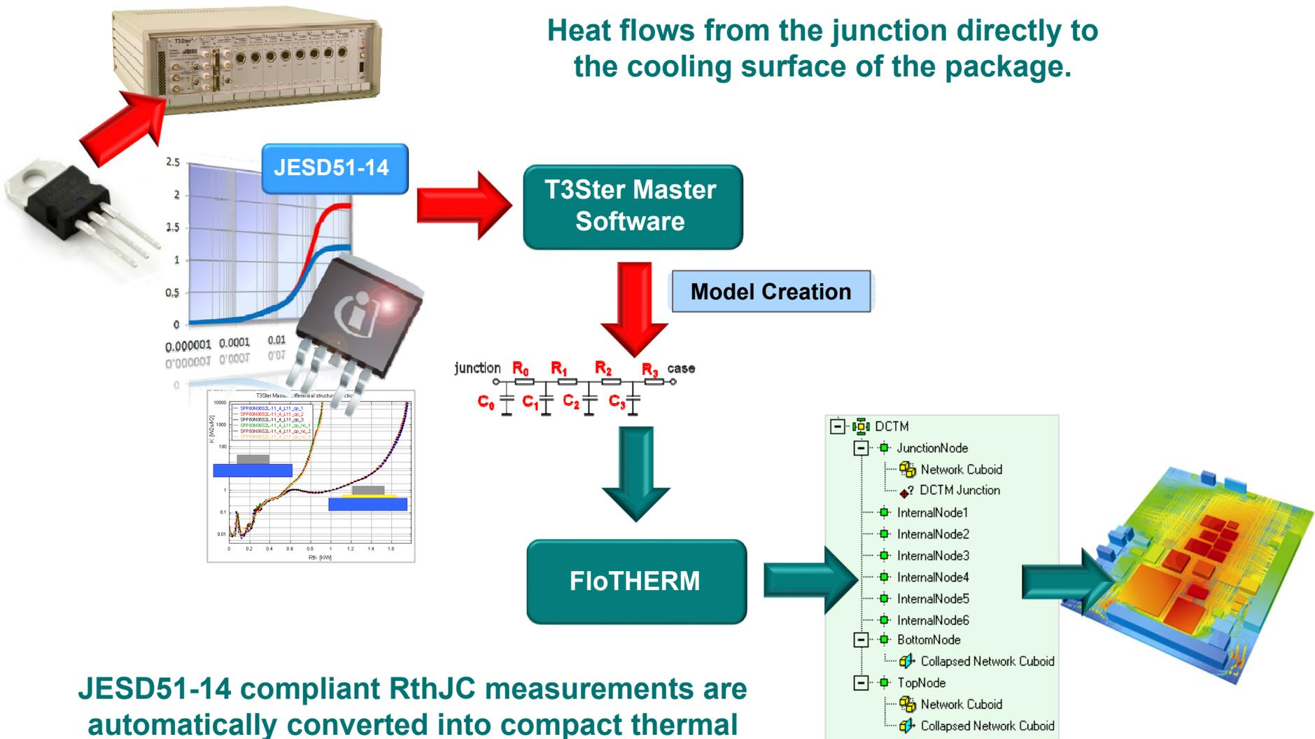
JESD51-14 compliant  $R_{thJC}$  measurements are automatically converted into compact thermal models used in FloTHERM.
