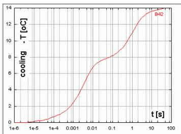
Structure functions for test based compact model generation
