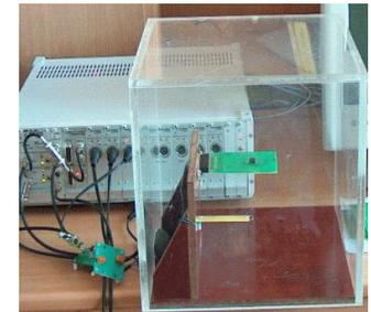
Majority of the  $R_{thja}$  is caused by the JEDEC standard test environment.
