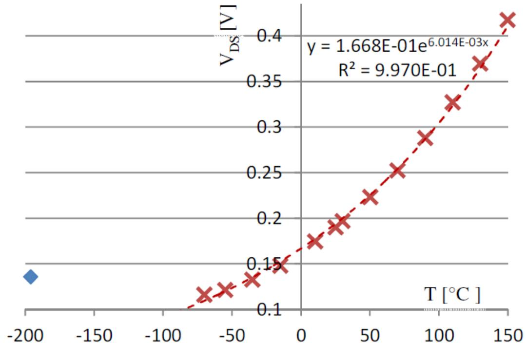
**Figure 5: RDS calibration curve of the depletion device with exponential regression, at 0.5A measurement current**
