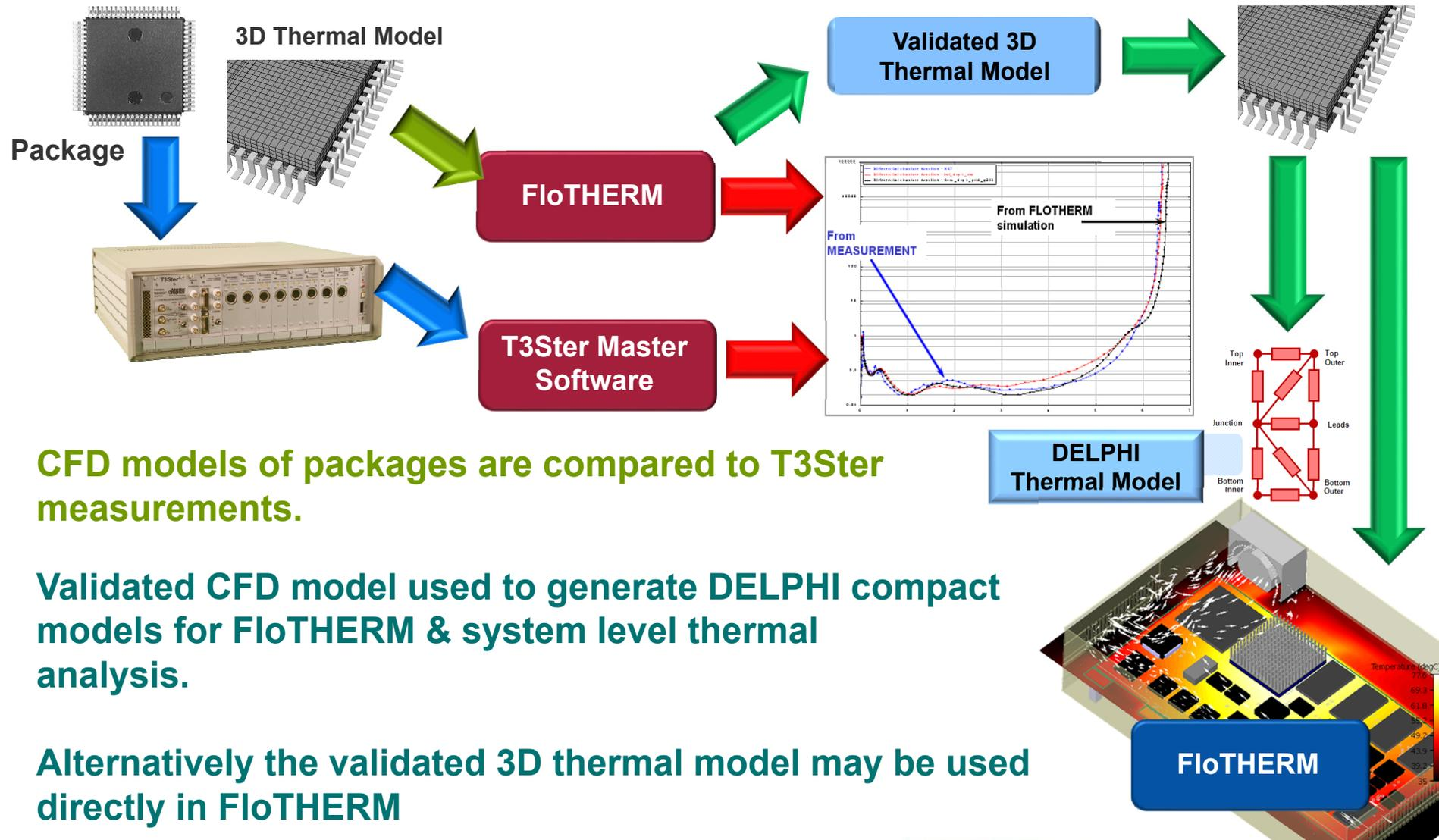
CFD models of packages are compared to T3Ster measurements.
