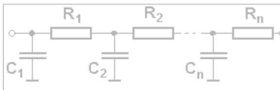
This model structure is characteristic to power semiconductor packages
