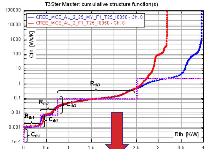
A simple model can be created, suitable even for hand calculations.
