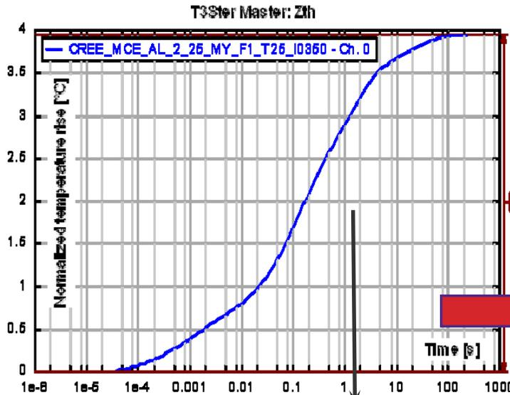
At higher frequency the absolute value of  $Z_{th}(\omega)$  is smaller:
