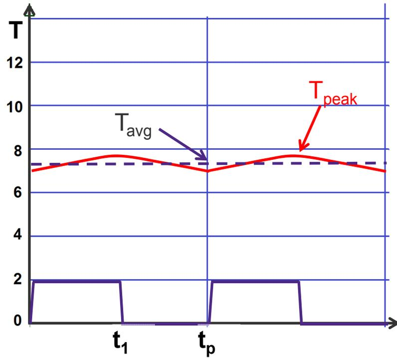
$t_1=0.1\text{ms}$ ,  $t_p=0.2\text{ms}$ ,  $\delta=0.5$ ,  $f=1/t_p=5\text{kHz}$ ,
