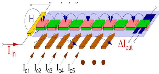
Fig. 13. A sketch showing multiphase clocking wires underneath the field-coupled inverter structure [40].
