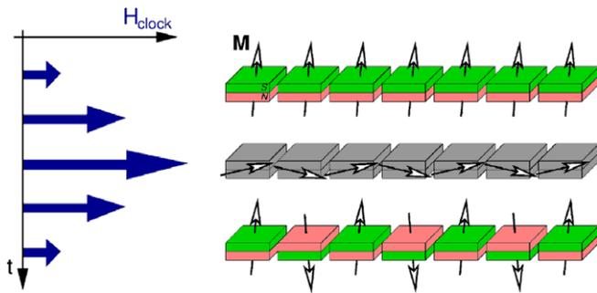
Fig. 14. Magnetization distribution in a ferromagnetic quantum cellular inverter gate at three different points in time (from [40]).
