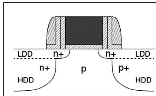
Fig. 7. Butted source contact MOSFET.
