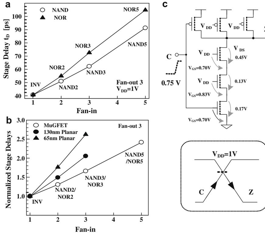
Fig. 3. Stage delays of complex MuGFET CMOS gates (a) and comparison of average stage delays to planar CMOS gates (b) for increasing fan-in. MuGFETs are based on single-midgap metal gate with symmetric threshold voltages. A snapshot of a NAND3 operation during the rising input transition is shown in (c) (from [11]).
