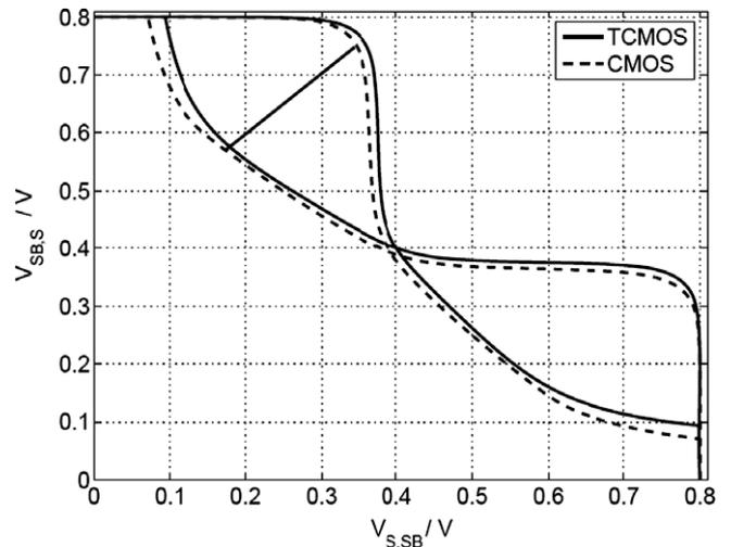
Fig. 10. Comparison of static noise margin of SRAM cells with conventional CMOS transistors and TFETs as pull down devices.
