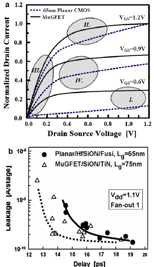
Fig. 2. MuGFET and planar MOSFET characteristics: (a) drain current and (b) inverter delay-leakage trade-off (from [8]).
