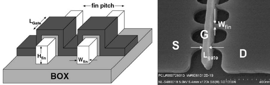
Fig. 1. Schematic view (left) and SEM picture of MuGFET [8].
