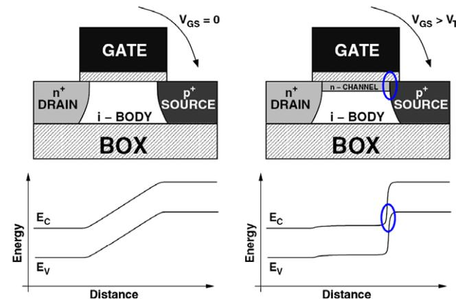
Fig. 5. 2D Cross-section of an SOI Tunneling Field Effect Transistor and band diagrams for OFF and ON states [23].
