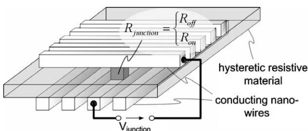
Fig. 11. Crossbar architecture of programmable nanodevices connected by nano-wires (reprinted from [36]).
