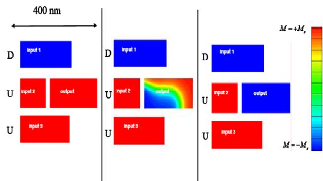
Fig. 12. Simulation results for the magnetic switching behaviour of a quantum cellular automata majority gate [38].
