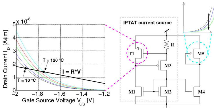
Fig. 8. Schematic of proposed voltage reference circuit combining a TMuGFET T1 with five MuGFETs M1–M5 [23].
