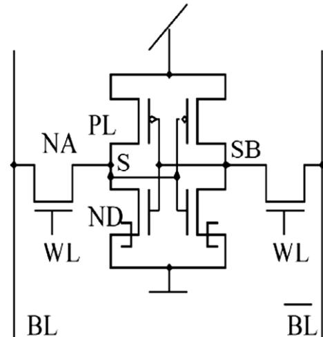
Fig. 9. Static memory cell with two NMOS, two PMOS and two TFET transistors.
