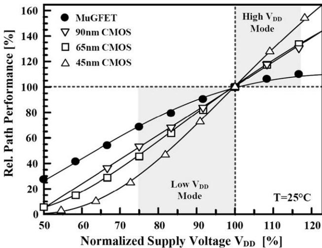
Fig. 4. Comparison of voltage scaling efficiency in planar and MuGFET technologies (after [18]).
