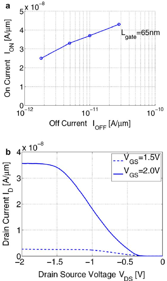
Fig. 6. On- versus off-current for different channel lengths ( $L_{gate} = 65$  nm, 80 nm, 120 nm, 500 nm) (a) and ID–VGS characteristics of 65 nm p-type MuGFET (b) (from [23]).
