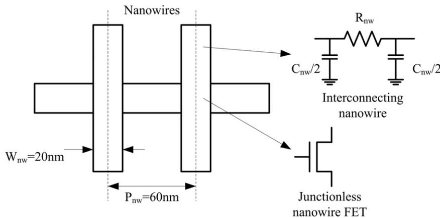
**Fig. 14.** Geometry and modeling of the nanowire crossbar.
