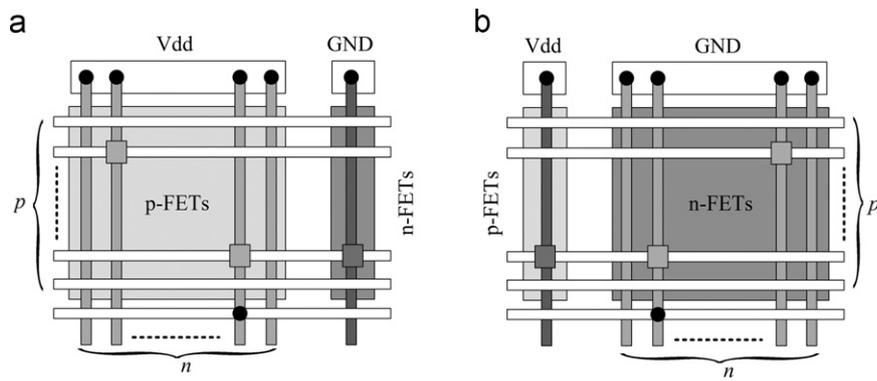
Fig. 12. Asymmetric nano architecture, (a) NAND-based structure, (b) NOR-based structure.
