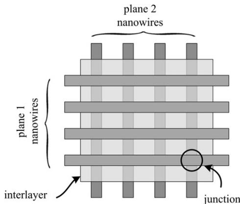
Fig. 2. Schematic view of a nanowire crossbar.
