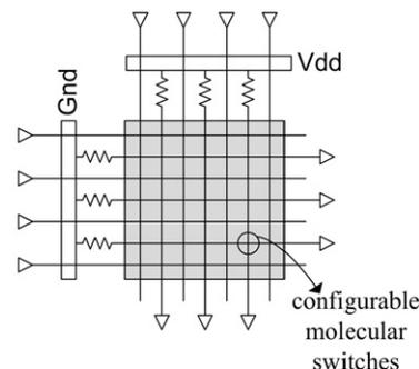
fabric is built up as a crossbar silicon nanowire grid with crossed nanowire field-effect transistors (xnwFETs) at certain crosspoints (Fig. 6). The channel of an xnwFET is aligned along one NW while the perpendicular NW above it, acts as a gate. Each basic block can be
