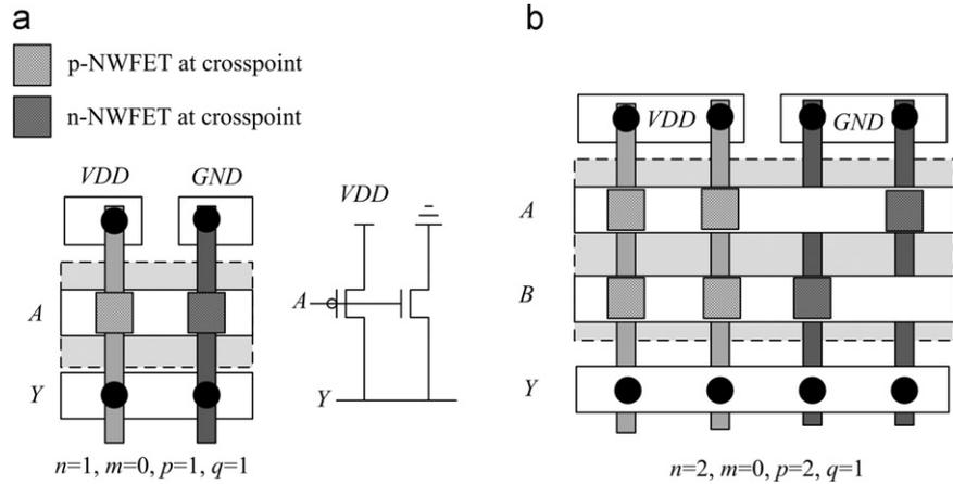
Fig. 11. Logic gate implementation using nanowire crossbar, (a) inverter and its equivalent circuit, (b) 2-input NOR gate (reproduced from Ref. [26]).
