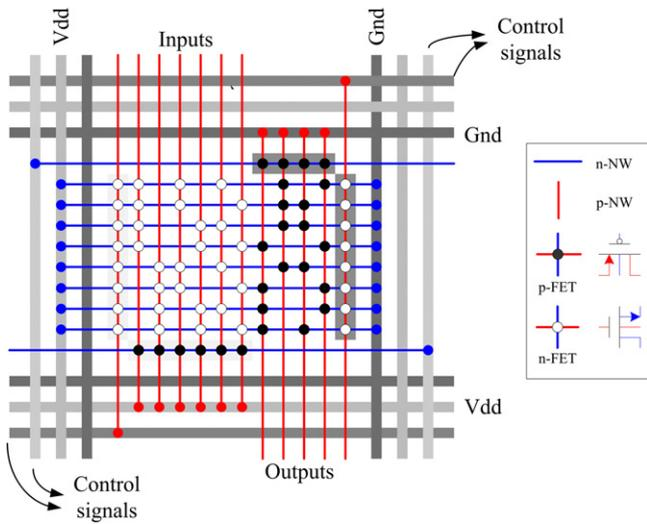
Fig. 6. NASIC building block (reproduced from Ref. [52]).
