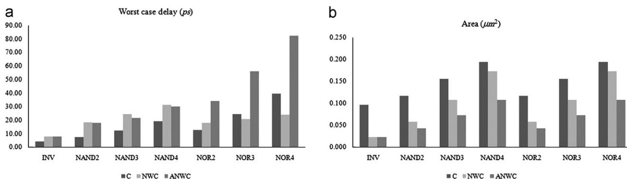
Fig. 15. Simulation results of basic logic gates, (a) worst case delay, (b) gate area.
