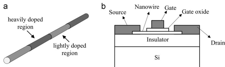
Fig. 1. (a) Encoded nanowire, (b) Schematic of a NW-FET device with high- $\kappa$  dielectric layer.
