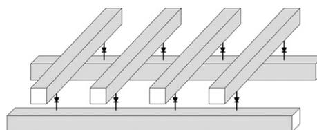
Fig. 9. (a) Schematic view of memristor [57], (b) memristor based crossbar with serial diodes.
