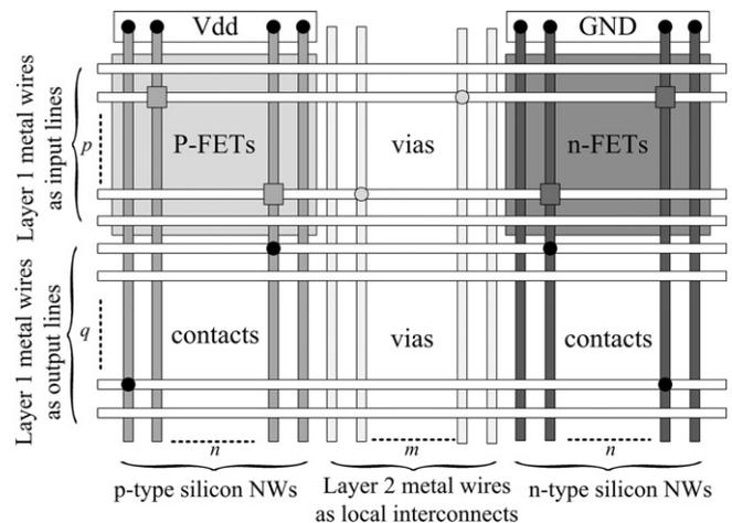
Fig. 10. FET-based crossbar architecture (reproduced from Ref. [26]).
