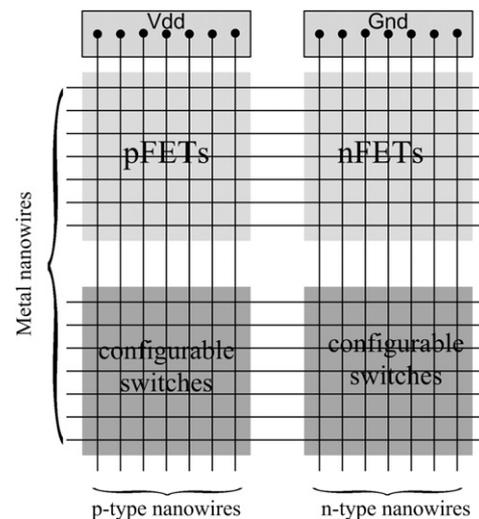
Fig. 5. Basic block of CMOS-like architecture (reproduced from Ref. [24]).
