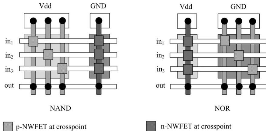
Fig. 13. Logic gate implementation using asymmetric nano-crossbar.
