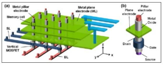
*Figure PIDS16* Schematic view of (a) 3D cross-point architecture using a vertical RRAM cell and (b) a vertical MOSFET transistor as the bit-line selector to enable the random access capability of individual cells in the array [60].
