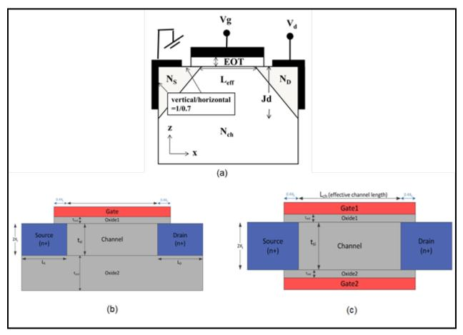
Figure PIDS1 Transistor Structures used for Simulations: (a) Bulk, (b) SOI, (c) MG
