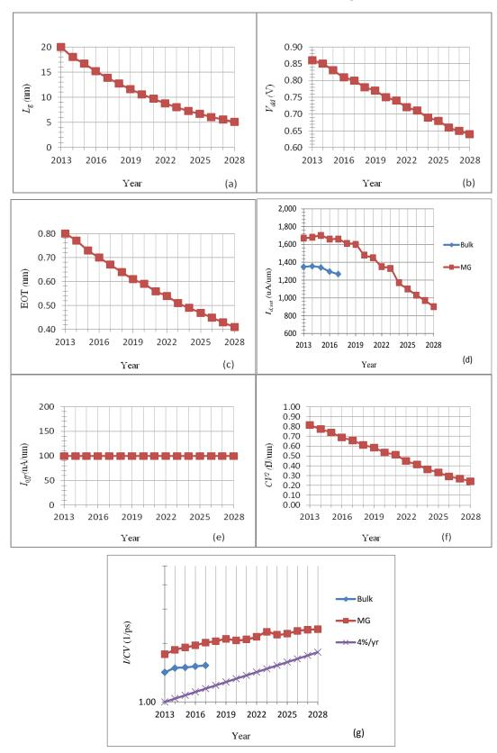
*Figure PIDS2* Scaling Trend of Logic HP Transistors. (a) Gate length, (b) Supply voltage, (c) EOT, (d) On-current Id, sat, (e) Off-current Ioff, (f) Dynamic power CV2, and (g) Intrinsic speed (I/CV)
