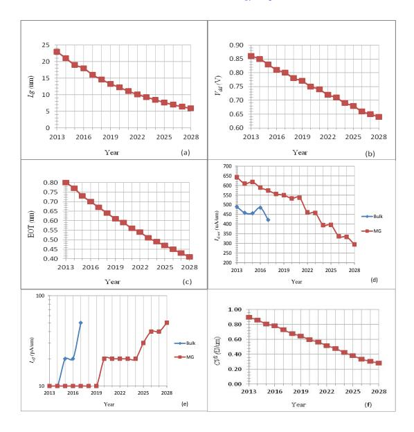
Figure PIDS3 Scaling Trend of Logic LP Transistors. (a) Gate length, (b) Supply voltage, (c) EOT, (d) On-current Id, sat, (e) Off-current Ioff, (f) Dynamic power CV2 and (continued on next page)
