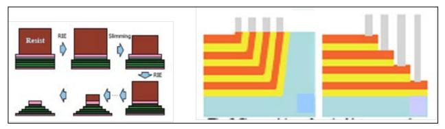
Figure PIDS15 (left) Scheme to make staircase landing pads for all layers by trimming one single layer of photoresist [42]. (right) A scheme to make contacts using tapered deposition and surface contact. Left: surface contacts are made in one operation. Right: conventional staircase contacts [44].
