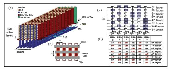
Figure PIDS11 A Vertical Gate 3D NAND Array with Decoding Method [45]
