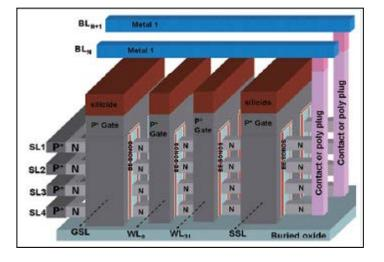
Figure PIDS12 Schematic Diagram of the PN Diode Decoded Vertical Gate (VG) 3D NAND Architecture. PN diodes are formed self-aligned at the source side of the VG NAND. Source lines (SL) of each memory layer are separately decoded, while WL, Bit line (BL), SSL and GSL are common vertically for the multi-layer stacks. Note that there is only one SSL and one GSL in one block [47].
