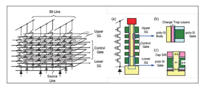
*Figure PIDS7* (*left) A 3D NAND Array based on a Vertical Channel Architecture [42]. (right) BiCS (Bit Cost Scalable) – a 3D NAND structure using a punch and plug process [42].*
