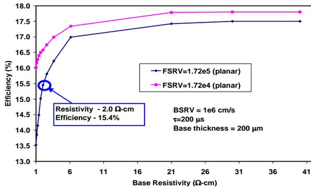
**Fig. 1:** PC1D model calculation showing efficiency of Al back junction cells as a function of base resistivity and front surface recombination velocity.
