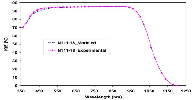
Fig. 5: Measured and simulated Internal quantum efficiency over the entire wavelength for the <111> n-type Al back junction solar cells.
