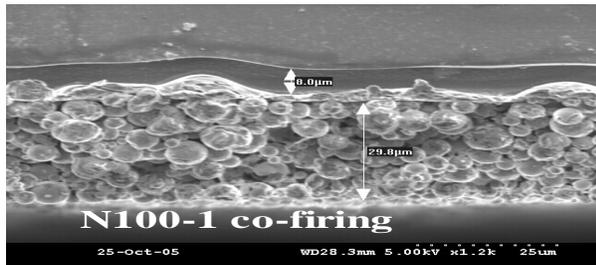
Fig. 4c: SEM micrograph of Al/Si interface in Al back junction cell on <100> (Frittled Al paste)
