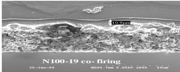
Fig. 4a: SEM micrograph of Al/Si interface in Al back junction cell on <100> (Frittless Al paste)
