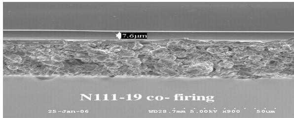
Fig. 4b: SEM micrograph of Al/Si interface in Al back junction cell on <111> (Frittless Al paste)
