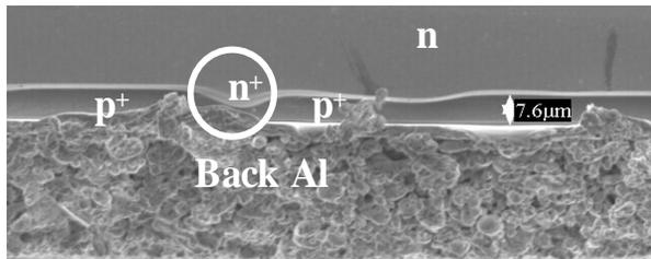
**Fig. 2:** Structure of Al back junction solar cell with a non p-n junction region.
