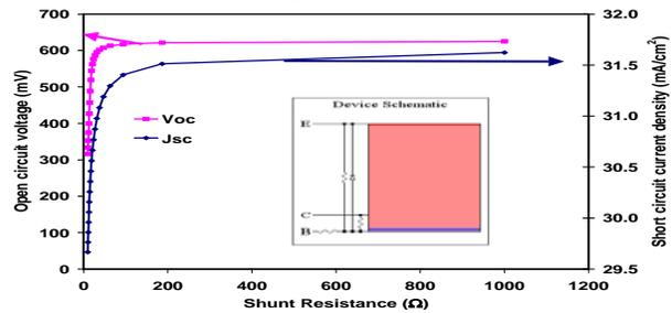
**Fig. 3:** PC1D model calculations and equivalent circuit for modeling low shunt resistance in n-base cells.
