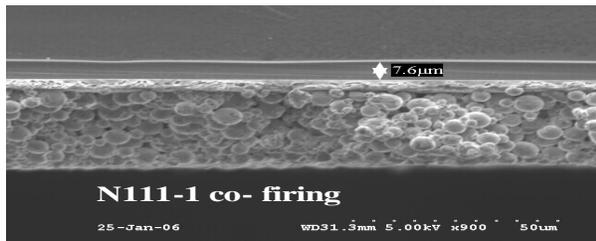
Fig. 4d: Frittled Al paste SEM on <111> Al back cell
