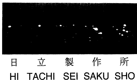
Fig.6 Kanji characters written by the NFTI method, which read Hi-Tachi-Sei-Saku-Sho (Hitachi, Ltd.). Each character is made up of a 16x16 dot nano needle structures.
