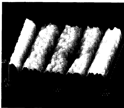
Fig.4 Beam Assisted Scanning Tunneling Microscope (BASTM) observation of a 100 nm line and space patterns formed in a 10 nm thick silicon dioxide layer, thermally grown on silicon substrate with 10 nm diameter resist dots : schematic figure (top) and BASTM micrograph (bottom)
