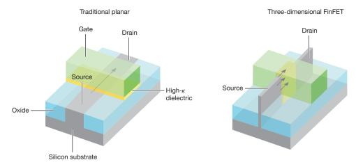
Figure 4 | FinFET transistors possess a much wider gate dielectric layer (surrounding the fin shape) than do MOSFET transistors and can use multiple fins.
